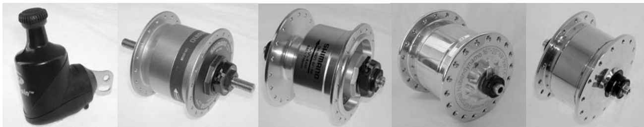
Fig. 2: Modern generators (from l. to r.): Lightspin, Shimano DH-3N30, Shimano DH-3N71, SON28/20, SON XS (see sidebar on p. 29)
